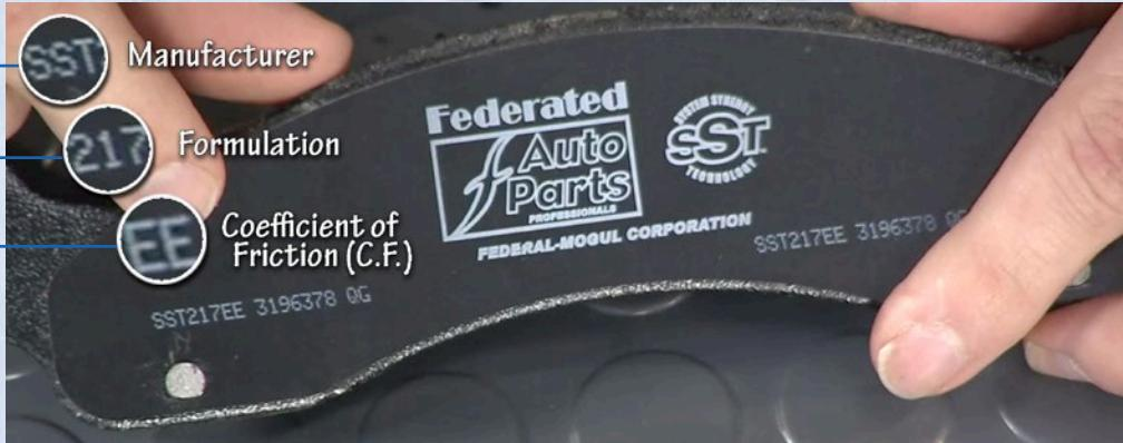
Brake Edge Codes can be found on the edge of the friction material or on the backing plate of every brake pad, along with some other codes. In this bulletin, we primarily focus on the final two letters, but here is an example of what the code consists of:
